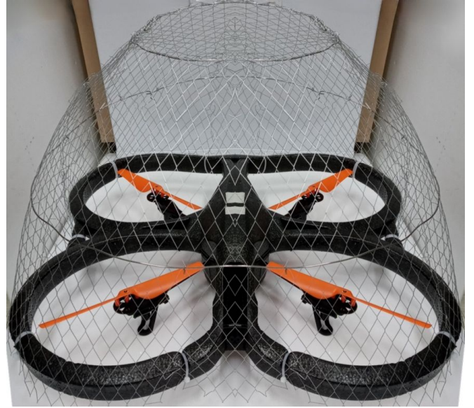
Fig. 1. Proposed Dome-shaped Haptic Drone (DSHD). A Haptic interface for 3DOF kinesthetic haptic feedback.
