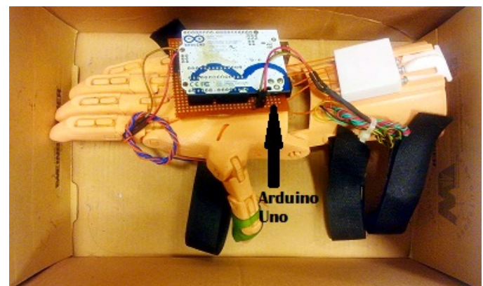
Fig. 2. Arduino uno screwed on the back of palm
