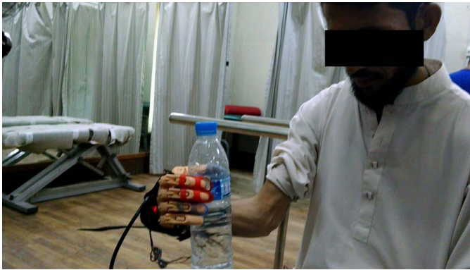
Fig. 15. Subject holding bottle with prosthetic hand consisting vibrotactile stimulation system
